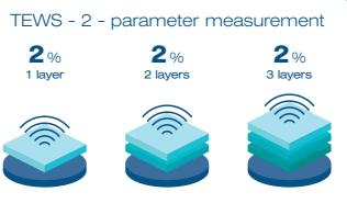
3 layers of same material show the same moisture, the density is recognized and moisture result compensated  $\rightarrow$  **correct results**
