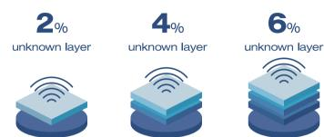
3 different layers of the same material with a typical 1 Parameter Method: Each layer increases the moisture  $\rightarrow$  misleading results
