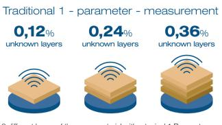
3 different layers of the same material with a typical 1 Parameter Method: Each layer increases the moisture  $\rightarrow$  **misleading results**
