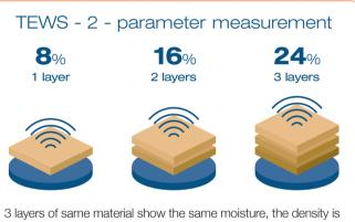
3 layers of same material show the same moisture, the density is recognized and moisture result compensated  $\rightarrow$  correct results
