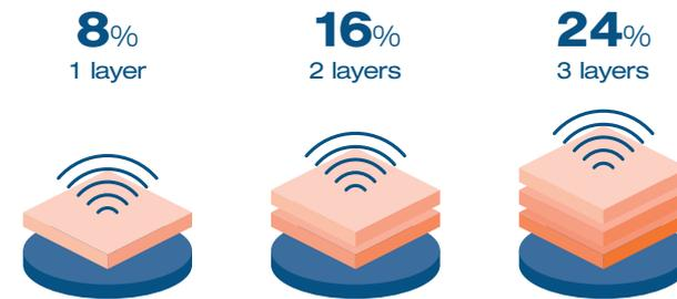
3 layers of same material show the same moisture, the density is recognized and moisture result compensated → **correct results**
