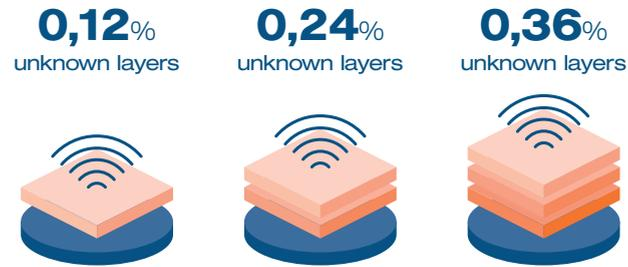
3 different layers of the same material with a typical 1 Parameter Method: Each layer increases the moisture → **misleading results**
