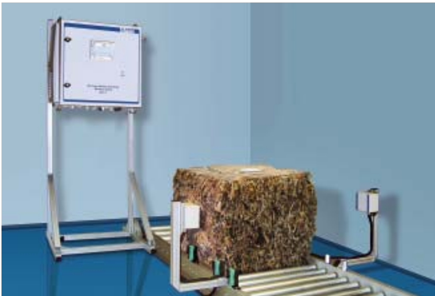
In-line moisture measurement of green leaf, cut tobacco and filter tow in bales and boxes – contact free and mass independent
